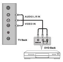
Connect the VIDEO and AUDIO output jack of the DVD or VCR to the AV IN jacks on the set using the RCA cable.
